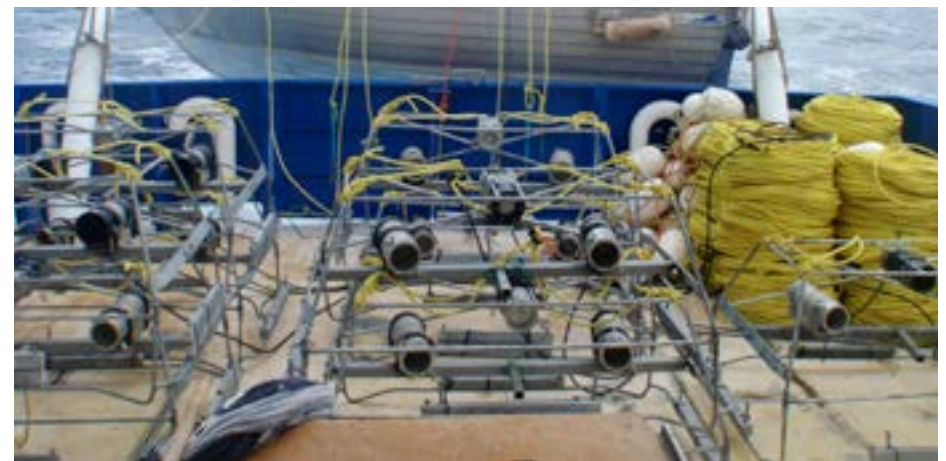
Stereo baited remote underwater video (BRUV) cameras about to be deployed.
