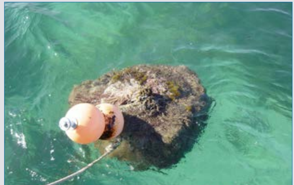
Artificial collector gathering puerulus samples.
